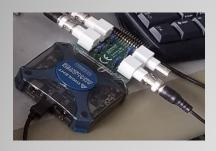
Digital/Analog I/O (NI/Digilent: \$279) + software (free) = oscilloscope, function generator, voltmeter, logger, spectrum analyzer, network analyzer ...
